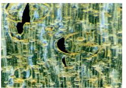
Micrograph of a damage pattern caused by hail
