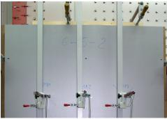
Facade panel at wind load test
