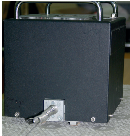
Determination of the slippery resistance of a resilient flooring according to EN 13893
