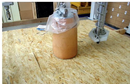
Impact test of load-bearing flooring
