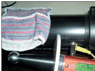
Measuring the charge transfer to evaluate the ignition hazard
